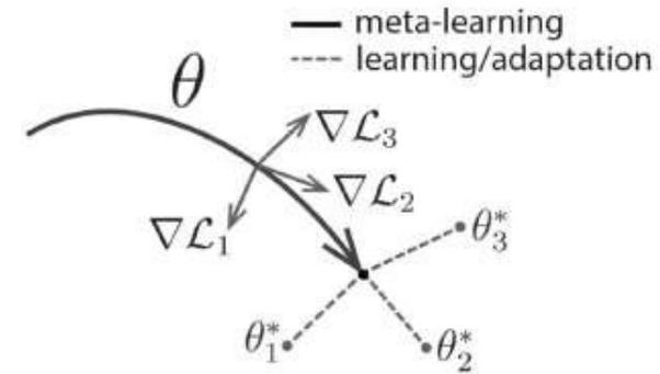
$$\theta \leftarrow \theta - \beta \sum_i \nabla_{\theta} \underbrace{\mathcal{L}(\theta - \alpha \nabla_{\theta} \mathcal{L}(\theta, \mathcal{D}_{\text{train}}^i), \mathcal{D}_{\text{test}}^i)}_{\text{"meta-loss" for task } i}$$
