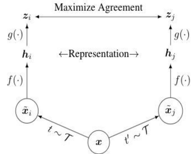
Figure 2. A framework for contrastive representation learning. Two separate stochastic data augmentations  $t, t' \sim \mathcal{T}$  are applied to each example to obtain two correlated views. A base encoder network  $f(\cdot)$  with a projection head  $g(\cdot)$  is trained to maximize agreement in *latent representations* via a contrastive loss.
